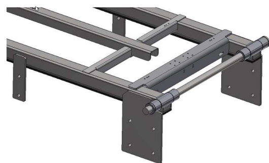
Figure 4 - Example installation of tipping pivot sleeves, reinforcing plates, mounting plates and cross-member
